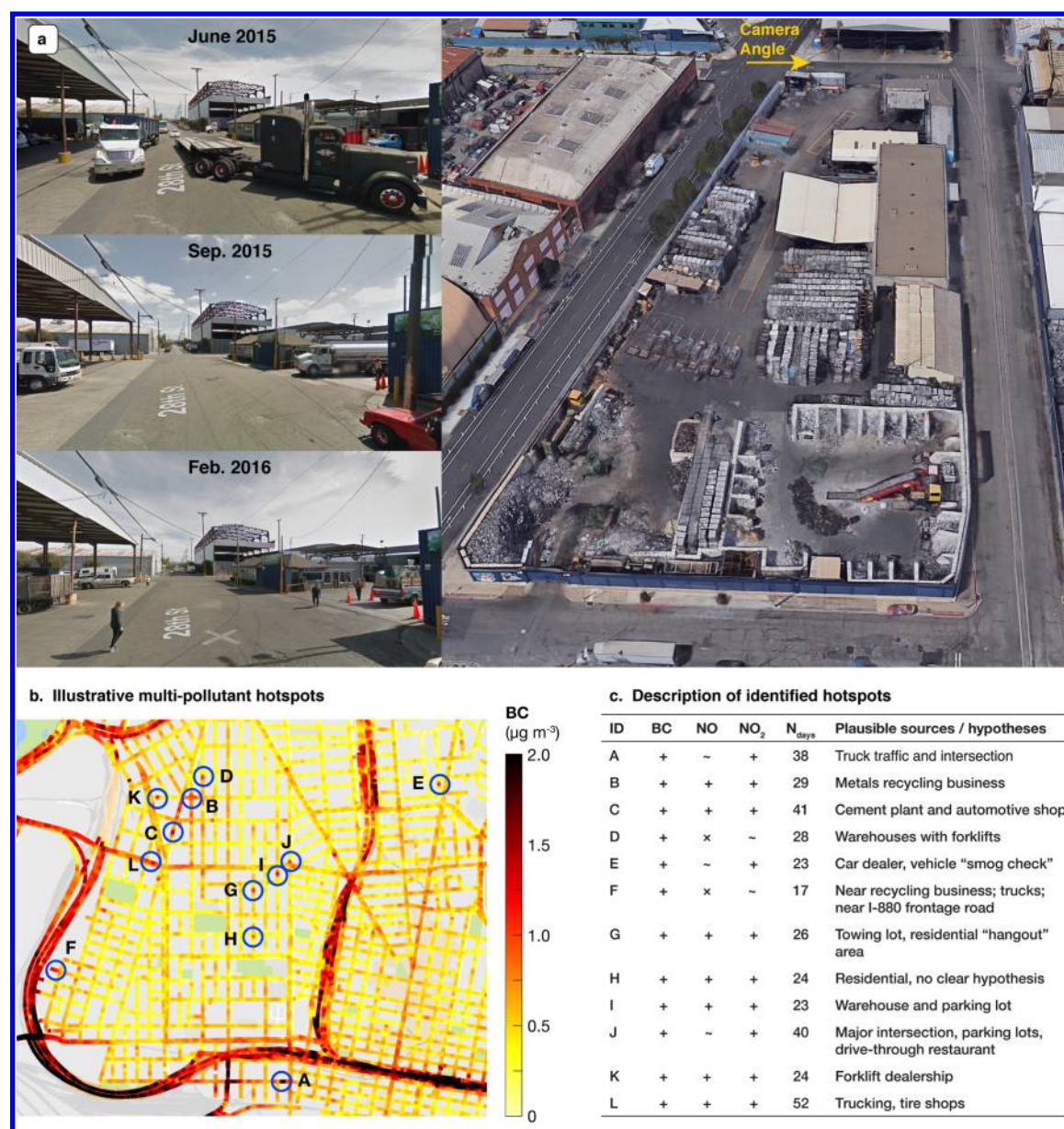
Figure 2. Illustrative pollution hotspots. a. Street View and aerial imagery of the metals recycling cluster highlighted in Figure 4a–c. Frequent heavy-duty and medium-duty truck traffic is evident in repeated Street View images. b,c. Multipollutant hotspots (i.e., prominent local concentration outliers) were identified from BC, NO, and NO 2 median concentrations as described in SI. Twelve illustrative hotspots labeled A–L here, overlaid on the 30 m BC map in b for context. List in c enumerates possible emissions sources for each illustrative hotspot, with the following classification scheme for each pollutant: (+) indicates a prominent localized hotspot or cluster of roads where concentrations are sharply elevated above nearby background levels, (∼) indicates a less prominent hotspot or cluster with moderately elevated levels, and (x) indicates the absence of a clearly discernible hotspot. Imagery © 2016 Google, map data © 2016 Google.
